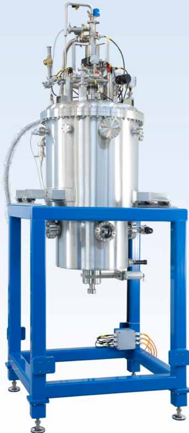
A 3-Axis superconducting magnet and UHV cryostat installed at the Diamond Light Source
