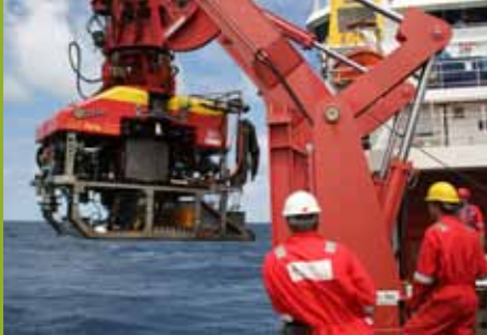
NOC – Isis is the UK's deepest diving remotely operated vehicle, working at depths of 6000m. It has provided footage of hydrothermal vents and the animals that inhabit them.
