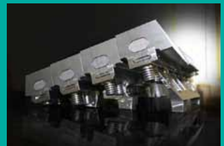
Left: A CAD image of the ITER like wall installed in JET. Above: Tungsten-LBSRP test array with Langmuir probes. Above right: MGS Vacuum Sinter facility. Right: Single Tungsten-LBSRP showing Inconel 625 wedge carrier and spring assembly. (Images courtesy of EFDA/CCFE and FZ Juelich)
