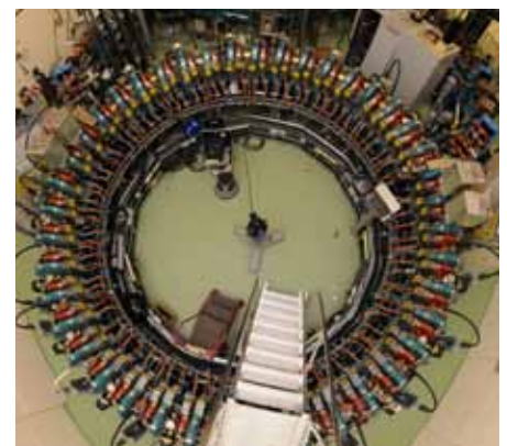
The pioneering EMMA (Electron Model for Many Applications) accelerator is a prototype for a brand new type of particle accelerator that will massively impact fundamental science by changing the way such accelerators across the world are designed and built in the future
