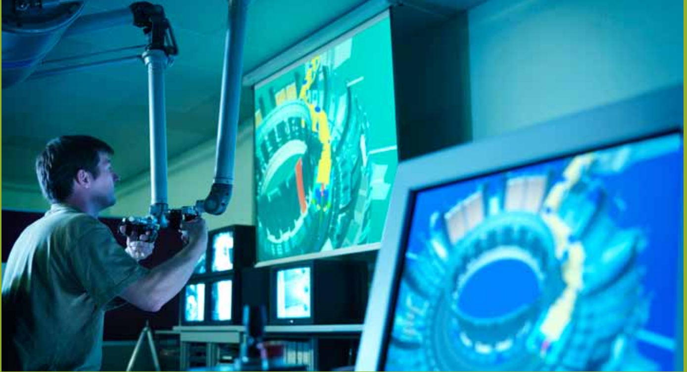
State-of-the-art remote handling technology is used to maintain and upgrade the JET facility. (Image Courtesy of EFDA-JET)
