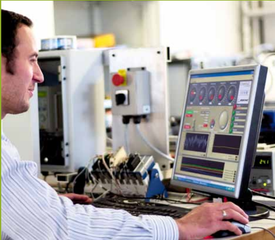
IVHM Centre – Left: Fuel rig experiment with National Instruments LabView interface. Top: Test workstation for Machine Fault Simulator & Wavelet transform method. Above: Testing and soldering of a test printed circuit board. Right: Machine Fault Simulator experiment
