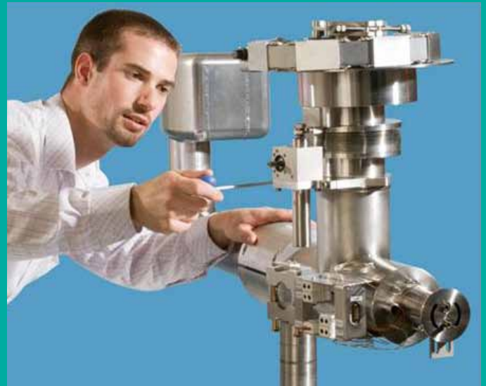
Inspection of a moderator for ISIS's new research facility, Target Station 2
