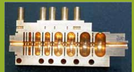
Above: A virtual computer-aided design of a compact microwave-driven linear electron accelerator system for X-ray scanning. Above right: A waveform showing the accelerating electromagnetic waves in the operating accelerator. Right: The detailed precision machining of the microwave linear accelerator waveguide at a high frequency of approximately 9 Gigahertz
