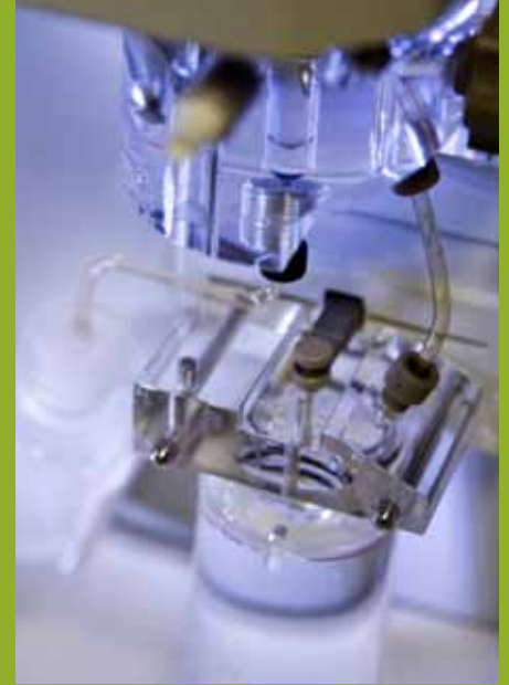
MRC Protein Phosphorylation Unit, Dundee (photography by Noel Murphy). DNA sequencing and DNA fragment size analysis (like "DNA fingerprinting")/Anode buffer and polymer assembly in Applied Biosystems model 3730 Genetic Analyzer
